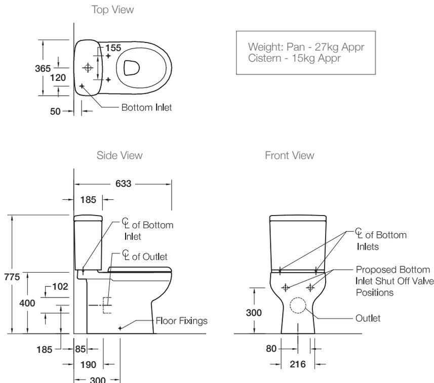
**Vario pan connector S-trap installation**
