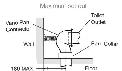
\*Note: Set outs between 180-220mm are achievable with the Long Adjustable Vario Connector 77837A-NA (not supplied).
